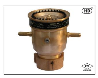
Clean the nozzle and reassemble. While re-assembling the nozzle or as a normal preventive maintenance, water proof lubricant must be used on seal and moving parts for smooth operation. The nozzle must be operated periodically under full flow straight stream and for fog pattern.
