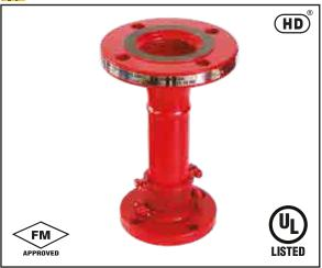
The inlet of foam maker is designed to create venturi jet which draws air into the foam solution stream. The air is drawn into the foam solution through holes located on the foam maker covered with stainless steel screen to exclude nesting birds and insects. The aerated foam is directed into the pourer for the gentle application of the expanded foam. The pourers are available in different models.
